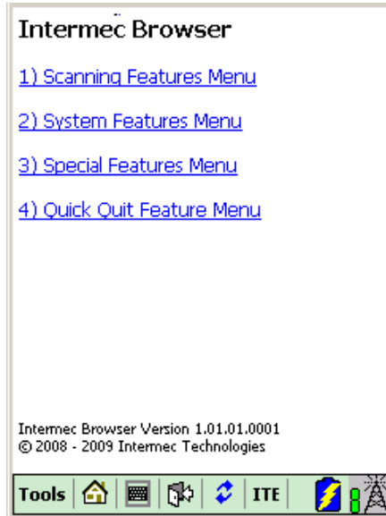
Use Intermecc Browser to directly configure and control the barcode scanner and to maintain complete control over the keyboard
